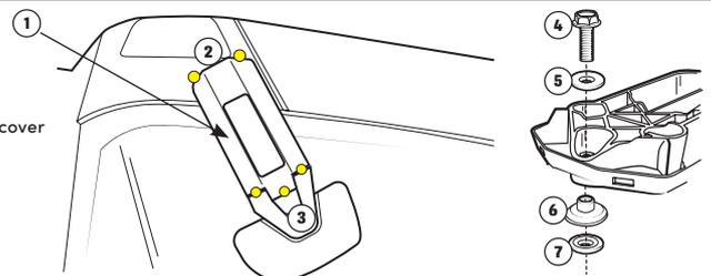
5. Place the mirror extender (1) on the front mirror with 3 carriage bolts (6), spacers (4), seals (5), with flat washers (3) and lock nuts (2).
