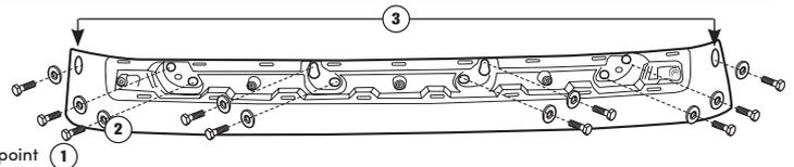
3. Seal the hole on the left exterior of the cabin no longer used attachment point (1). Repeat on the right side of the cabin external no longer used attachment point. On cabs with a high plastic front cover (2) can be ordered from your local Volvo workshop.
