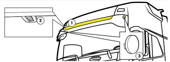
2. Remove the sunvisor from the cab by removing 10 flange screws (1) and washers (2).
