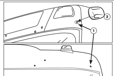
4. Remove the back cover of the front mirror (1), by first pushing in the two upper lockings (2), and then the three lower lockings (3).
