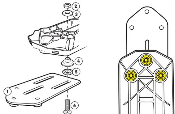
6. Apply a thin layer of sealant around the mounting holes for the front mirror on the cab (yellow marking).
