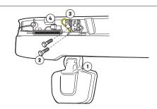
Remove the sunvisor from the cab by removing remaining 4 screws (1).
