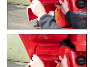
7. Angle the door extension so that the upper tape makes contact and press firmly for ~30 seconds.
