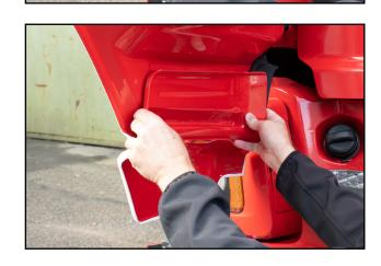
Check that the door extension moves freely from the step on the drivers side when tilting the cab. (When tilting the cab, the cab moves sideways. The distance between the door extension and the step will decrease) If the product is attached correctly you should have a clearance of approximately 5mm. If there's a problem. Redo the mounting procedure
